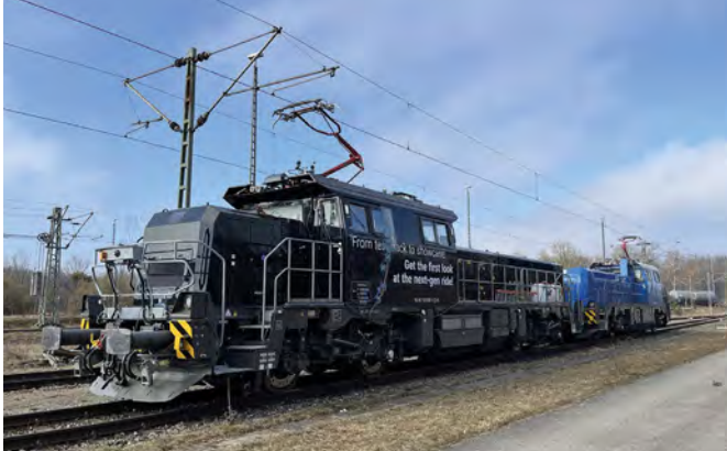
Die Hybridlokomotive Modula (Foto: Vossloh Rolling Stock).
